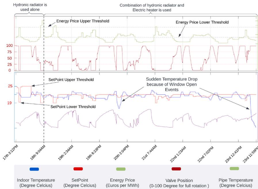
Fig. 5. The results of the local cloud-based DR optimization experiments for a space heating scenario in a smart home in Lulea, Sweden. We ran the experiments for seven days. The horizontal axis represents the timestamps, and multiple vertical axes show the indoor temperature, setpoint, energy prices, valve position, and radiator inlet pipe temperature curves.
