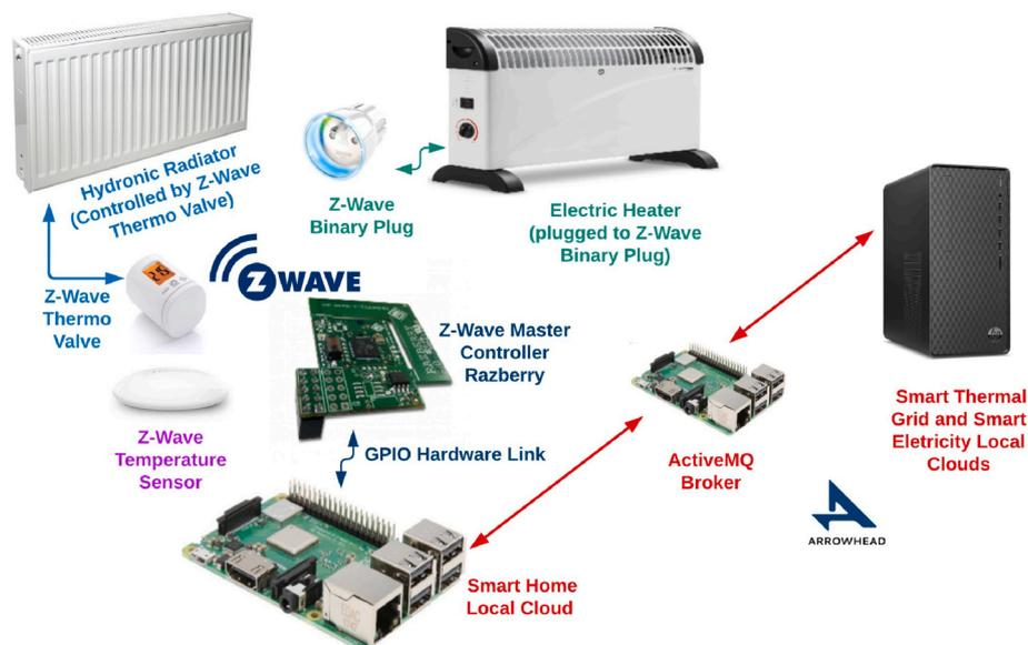
Fig. 4. The Hardware Setup for local cloud-based DR optimization experiment.
