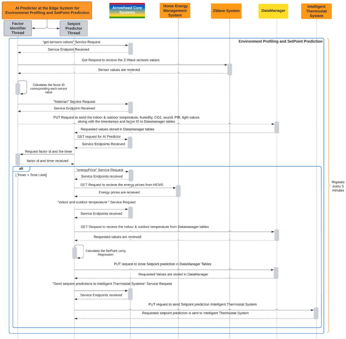
Fig. 7. Sequence diagram of environment profiling and setpoint prediction.
