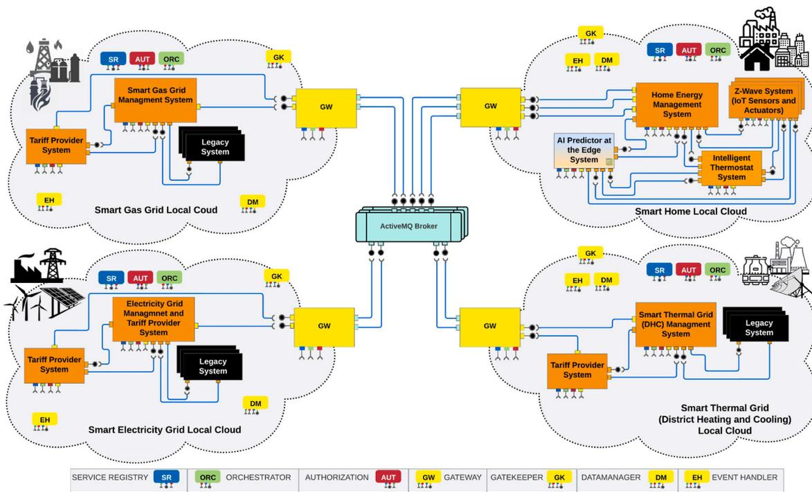
Fig. 3. The systems using Eclipse Arrowhead Local Cloud and Application Systems for the demonstration experiment.
