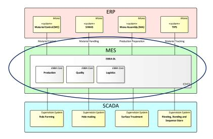
Computerized systems used in manufacturing, to track and document the transformation of raw materials to finished goods.
