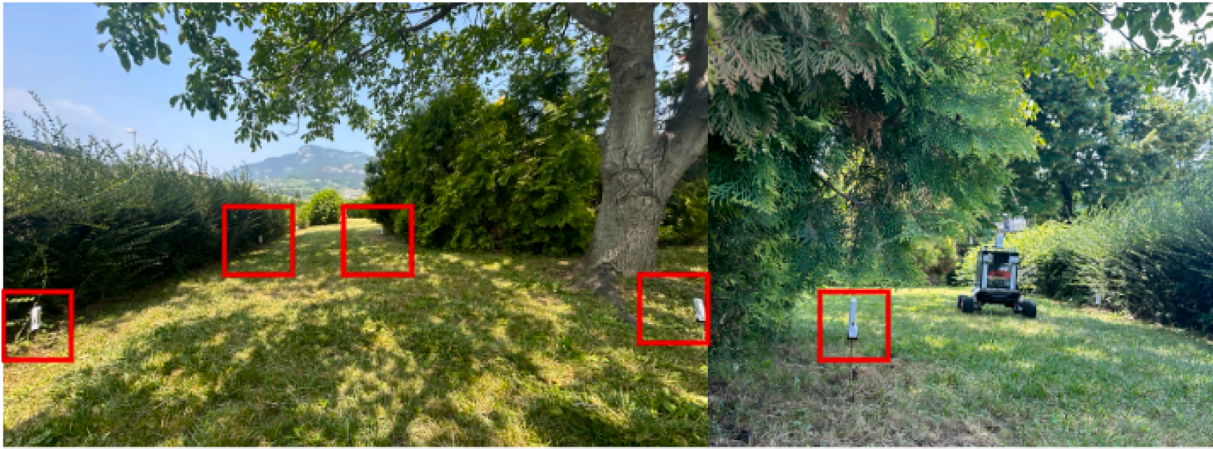
Fig. 6. The experimental setup used to assess the performance of the proposed adaptive EKF, with the UWB anchors clearly indicated in the red box. (For interpretation of the references to colour in this figure legend, the reader is referred to the web version of this article.)
